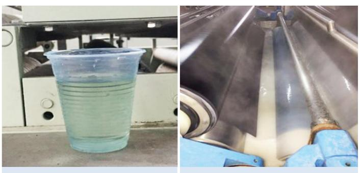
Sample of Waste Water Collected at Waste Drain after 15,000 Meters of Dyed Yarn
