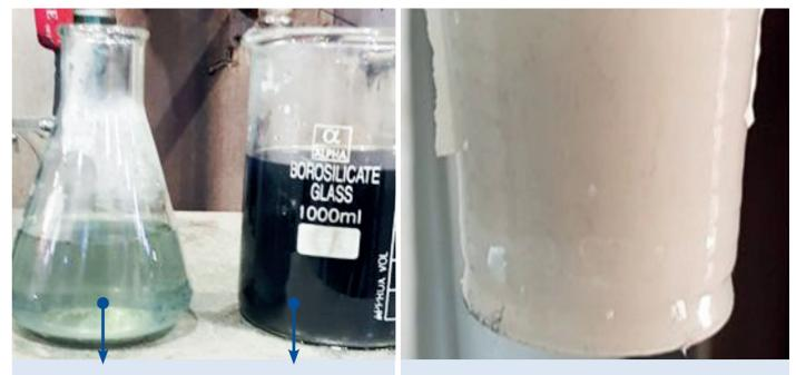
Waste Water from Indigo Wash Water Discharge after **BREVIOL® PROCESS**
